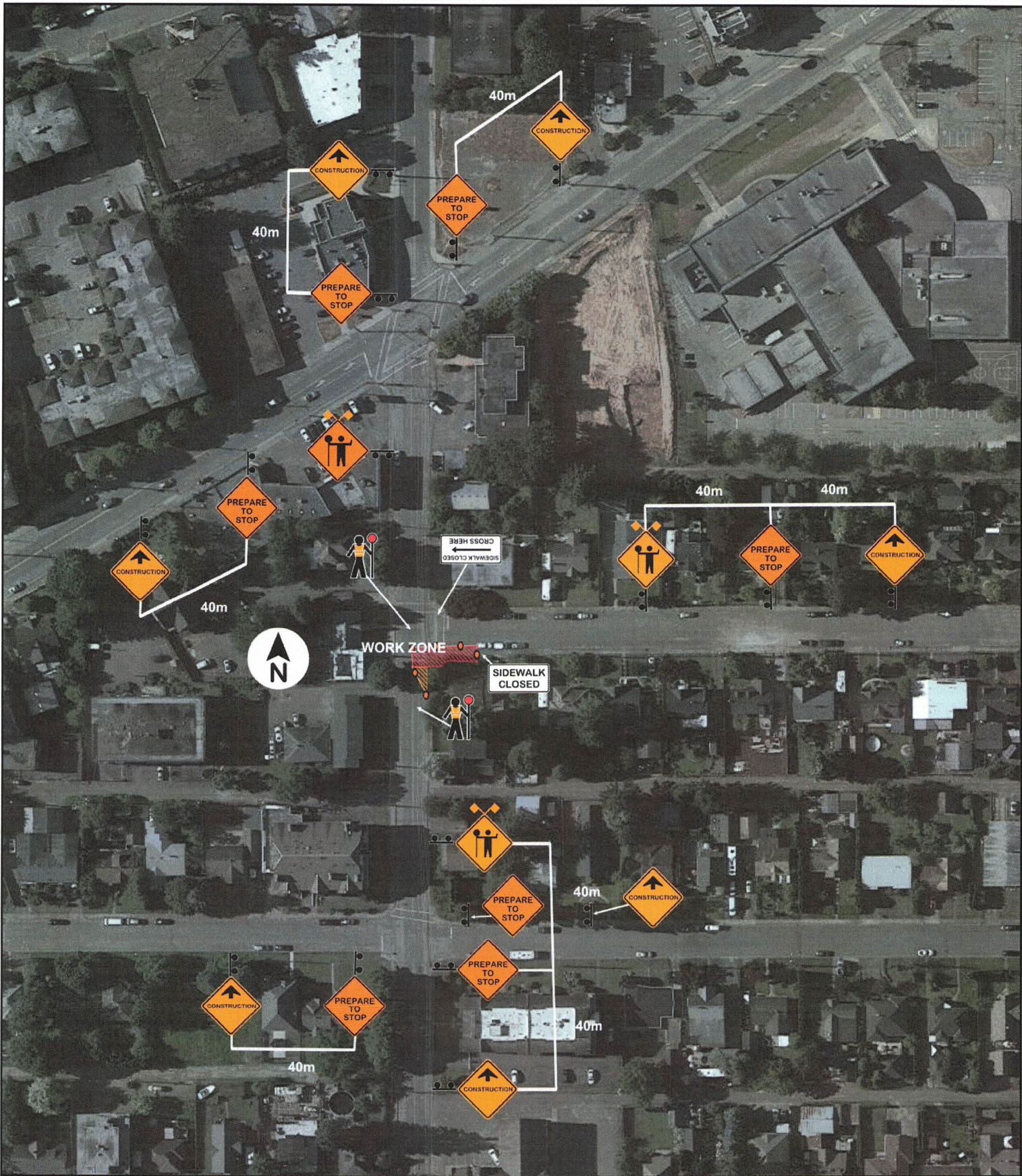
Figure 11.2: Intersection Lane Closure - Two-Lane, Two-Way Roadway with TCPs (Near Side) - Short and Long Duration TCPs on site to assist with vehicles, pedestrians, bicyclists and all others
